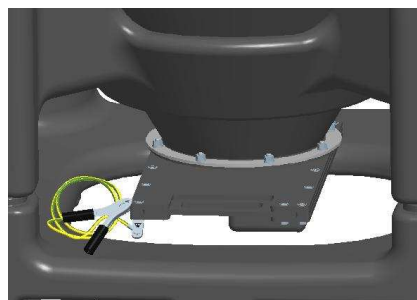
Horizontal outlet with 80mm SS316 butterfly valve
